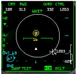
The ASEC will start to flash when the FCC calculates that the target is within missile manoeuvring and line-of-sight requirements. When the ASEC flashes, take it as a cue to fire. (Sorry I can't do a screenshot of it flashing! I would get complaints if it did not keep flashing after printing! ©)
