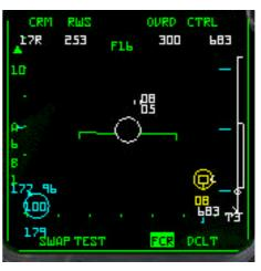
The ASEC will be at its largest when the contact is heading towards you. The chances of successful missile engagements are greater when you are head-on to your target and closure is high.
