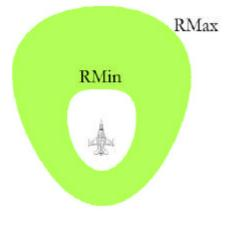
The first thing that needs to be understood when using any air to air missile is the concept of the weapon engagement zone (WEZ). The WEZ is the area around the target where the missile can reach and destroy the target. The diagram to the left shows an example WEZ for a nonmanoeuvring target. The AIM-120B has a maximum (RMax) and a minimum (RMin) firing range, the diagram represents the area between these two as a green 'doughnut'.
