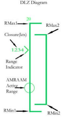
The Dynamic Launch Zone (DLZ) is a set of brackets on the side of the HUD and the Radar screen. The DLZ is comprised of two separate brackets, a distance indicator, and a closure meter. (Note the DLZ will only appear when you have a target selected). The diagram to the left labels the components of the DLZ.
