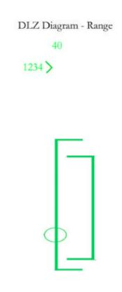
The numbers next to the range indicator are NOT the range. These numbers represent the closure rate of the target in knots. If there is a '-' in front of the number, the target is moving away from you. Finally with the DLZ is the AMRAAM Active Range. This little circle gives you am indication of how far away the AMRAAM will transition from inertial to active tracking. More on this later
